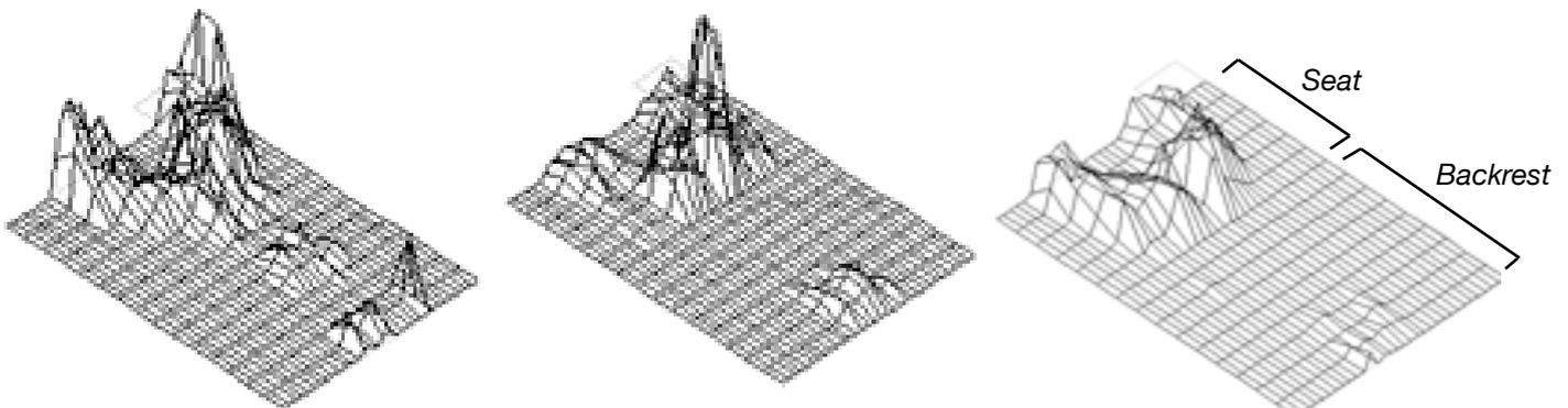
Pressure measurement chart on Premium chairs from two of the largest manufacturers in The Nordic region. The seat and backrest are indicated in the figure to the right
