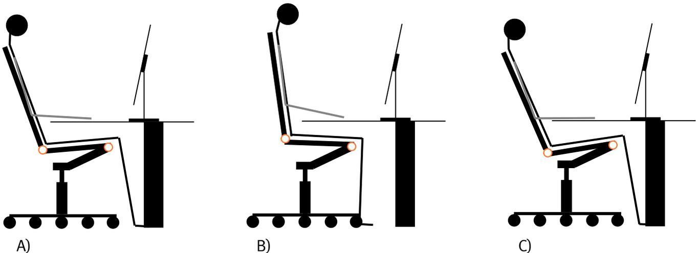
When you tilt forwards/backwards on a chair with a knee tilt or syncroglide mechanism, your backside moves up and down. Your hands, when they are placed as in the sketches, such as a keyboard, only move depthwise, instead of up and down. This is when your hands are also directly above the chair's knee joint. This provides a major advantage. We can sit in both forward and reclined workable sitting positions along with all positions in between the outermost positions.
